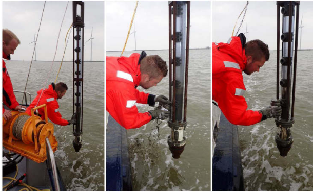
Figure 5. Taking fluid mud samples using the Sludge Sampler
